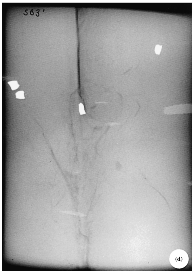
FIG. 7—Penetration of ballistic gelatin blocks at 3 ft (0.9 m) muzzle-to-target distance, showing (a) asterisk-shaped defect created by impacting sabot; (b) gelatin block bisected along slug track, demonstrating cavitation and radial extension of the slug nose fragments (arrows); (c) and (d) anterior-posterior and lateral radiographs of gelatin block demonstrating cavity and deposition of radiodense slug nose piece fragments in a radial fashion; and (e) projectile components recovered after firing, including four nose-piece fragments (upper right) from gelatin block, and slug base (upper left) and wads (lower) recovered from backstop.
